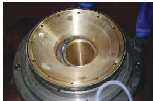
Large support area for the Head-Shaft enhances stability during operation
