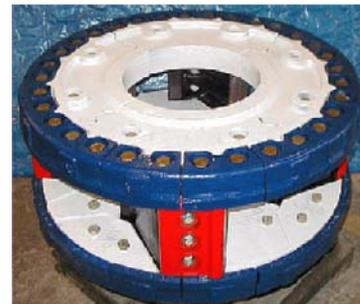
Clad Rotor for R-O-S configuration
