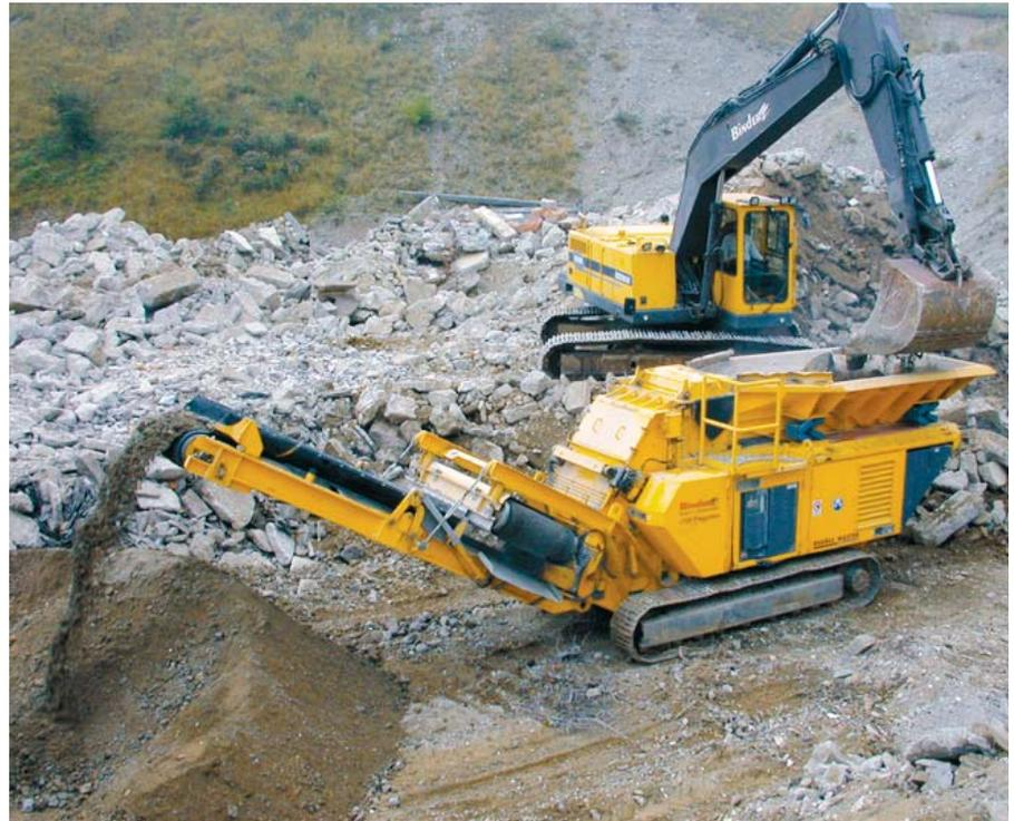
On-site mobile recycling can cut transport and create small cycles.
